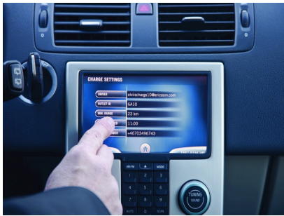
Figure 2. Illustration of the in-vehicle system that the driver uses to adjust current charge settings.
