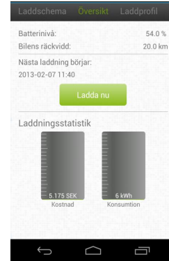
Figure 4. Illustration of the smart phone application. The user can access, via different tabs, charging schedule, and charge profile. The user can also decide to start the charging directly.
